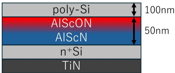
Fig.2 Si/AlScON structure used in this work.
