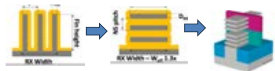
Fig.1: Evolution of nano-level LSI. From FinFET to CFET.
