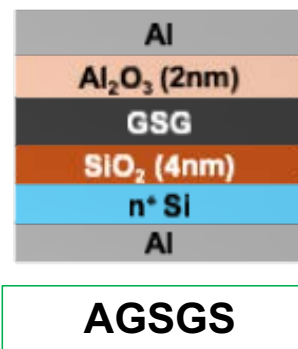
Fig. 6 Schematic of device structure for current suppression.
